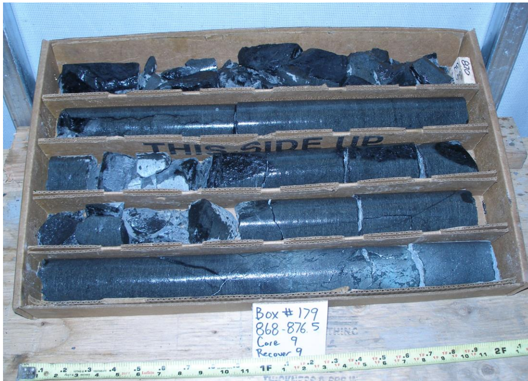
Figure 14: Broken and fractured basalt between 868' and 876.5'.
