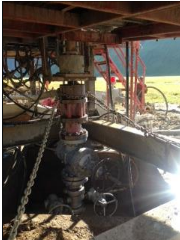
Figure 9: Wellhead configuration for the PQ section.
